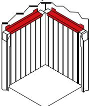
Fasten the mounting bracket to the firebox wall with screws.
